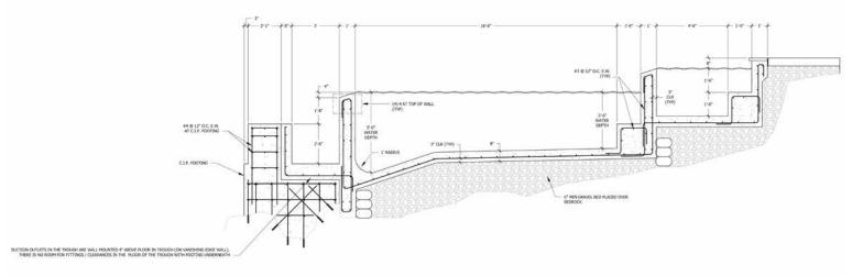
Fig. 2: Three-tier system of spa, main pool swimming area, and surge trough (Note: 1 in. = 25.4 mm)
