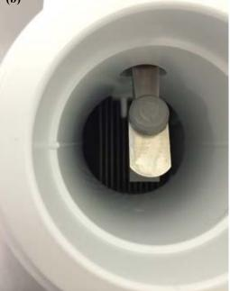
Fig. 3: Close-up views of a residential salt cell: (a) information it provides and the adjustments that can be made; and (b) close-up of the flow sensor which shuts the cell off when there is insufficient flow. Also shows the fins that provide the charges that separate the ions as the salt water passes through
