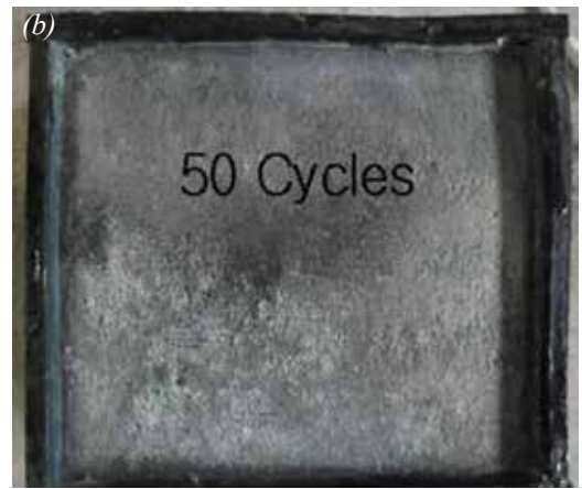
Fig. 6: Comparison of surface from surface scaling test: (a) before test; and (b) after 50 cycles
