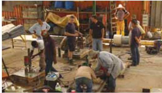
Fig. 6: Nozzleman coring the test panels
