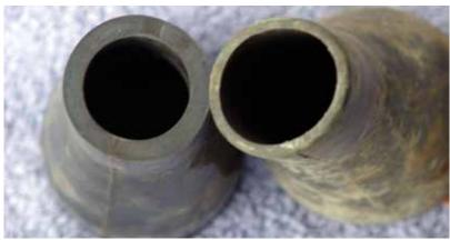
Fig 6: After placing only 80  $lb/yd^3$  (60 kg/m<sup>3</sup>), the worn tip on the right has become oversized and must be discarded
