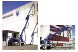
The Potenza is one of the better examples of a complete mobile unit for the spraying of shotcrete. This type of spraymobile has been setting the standard for shotcrete in tunnels and other areas of application using the wet-mix shotcrete method. They have become commonplace on many of the world's most important sites where sprayed shotcrete must be applied in large quantities without compromising quality.
