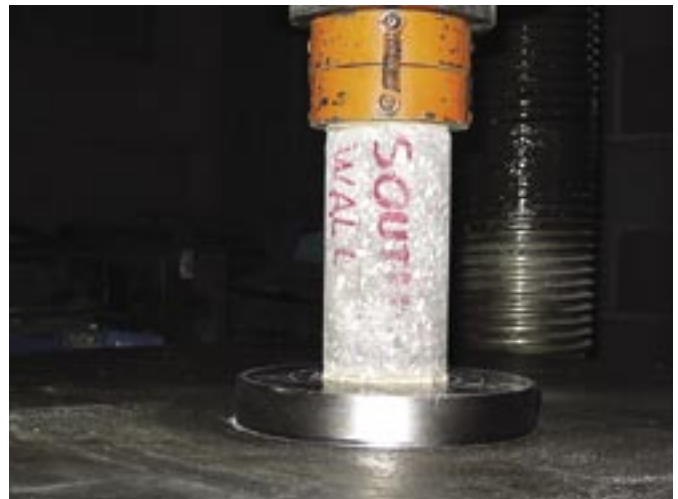
Fig. 2: Typical shotcrete core from pool during compression testing
