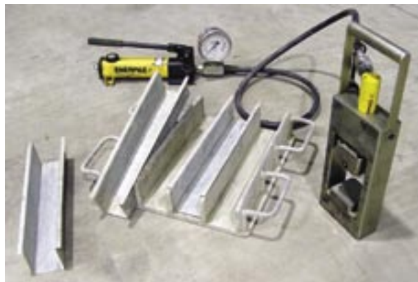
Fig. 3: Beam end tester (right) with mould and sheet steel inserts
