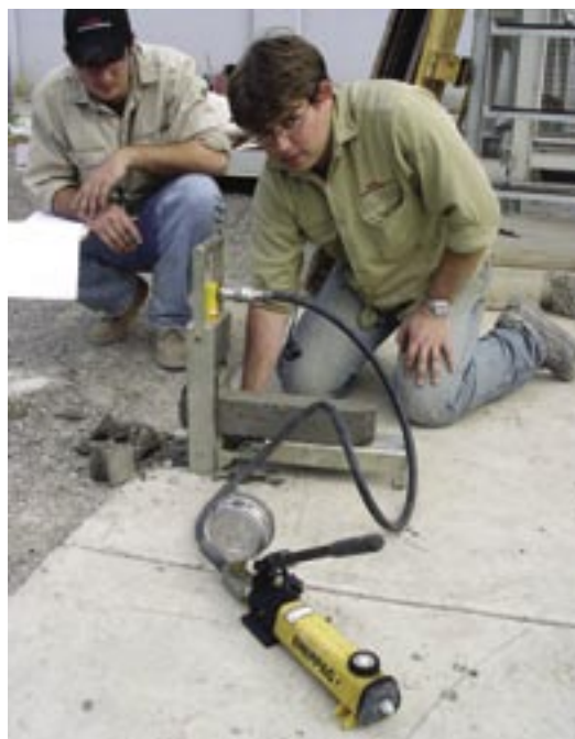
Fig. 4: Beam end tester in use
