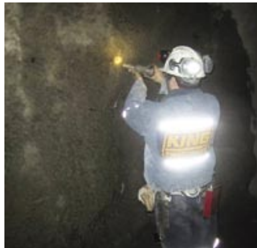
Fig. 3: Underground Schmidt Hammer testing
