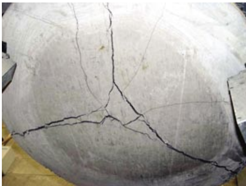
Fig. 3: Strain-hardening post-crack behavior of FRS ASTM C 1550 round panel containing 20.2 lb/yd 3 (12 kg/m 3 ) of Barchip Xtreme fiber showing the development of multiple cracks as a result of very effective redistribution of load. Normally, only three radial cracks form in this test
