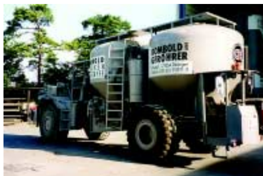
Figure 8: Double pressure cylinder on truck, with bottom-mounted batching screws (Rombold-Spritzmobil, 2002).
