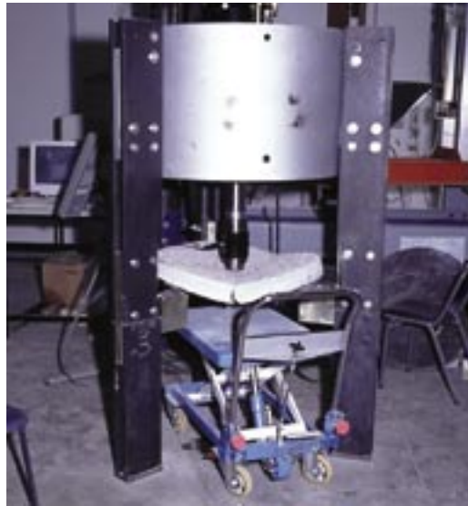
The Australian round panel test has proven to be a reliable QA tool and has been adopted by ASTM.
