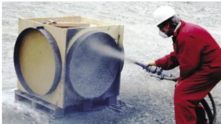
Figure 6: Round panel specimens being sprayed in Canada.
