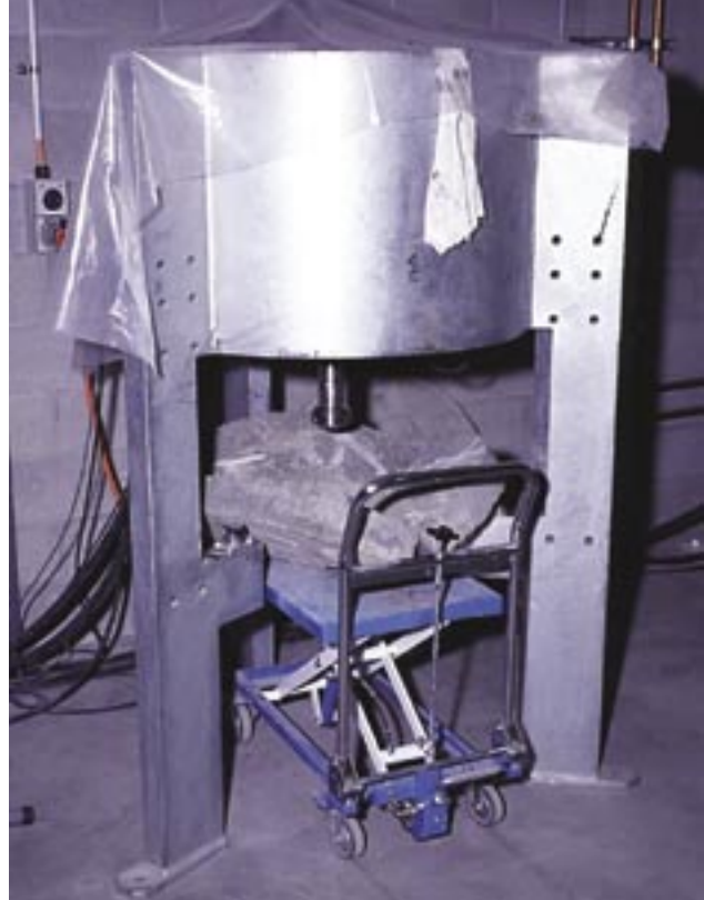
Figure 1: Round panel test rig with tested specimen.
