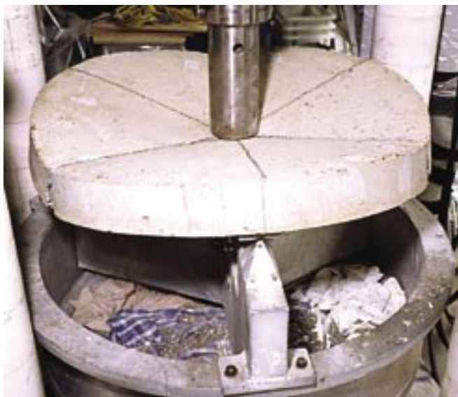
Figure 2: Alternative round panel test rig with specimen under test.
