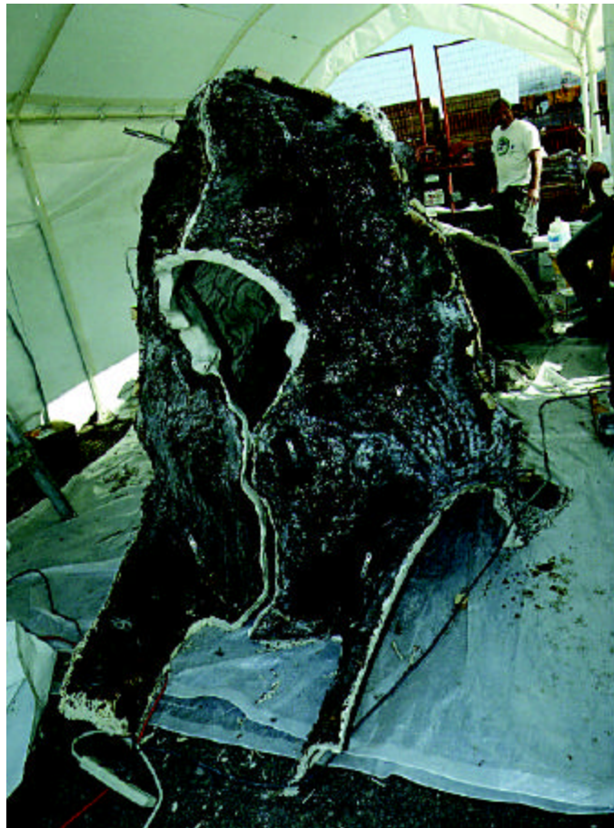
Figure 2: Rubber latex and glass fiber-reinforced resin mold stripped from original lion.
