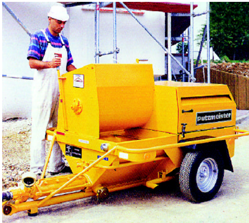
Figure 2: Typical worm pump (Putzmeister P11).
