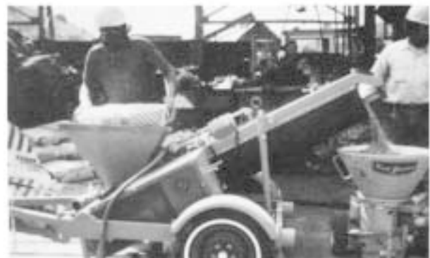
Figure 8: Mortar mixer with predampening assembly.
