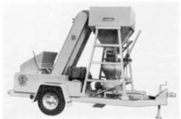
Figure 6: Mixing, predampening mixer with double chamber gun.
