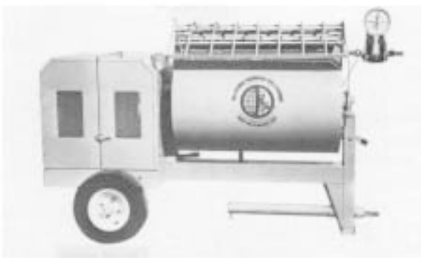
Figure 7: Mixing, predampening mixer with rotary gun.
