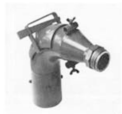
Figure 13: Casting head used in gun-casting.
