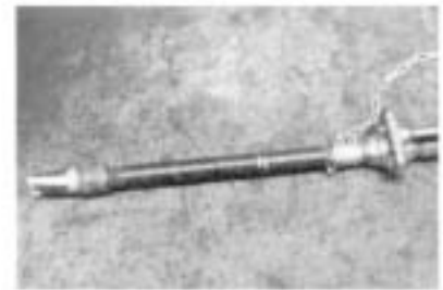
Figure 12: Hot gunning with special nozzle (lance).
