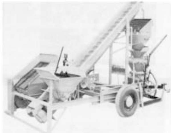
Figure 5: Proportioning, mixing, predampening mixer.
