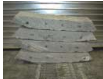
Figure 2: Certification panel used in the province of Quebec with typical sawed specimens.
