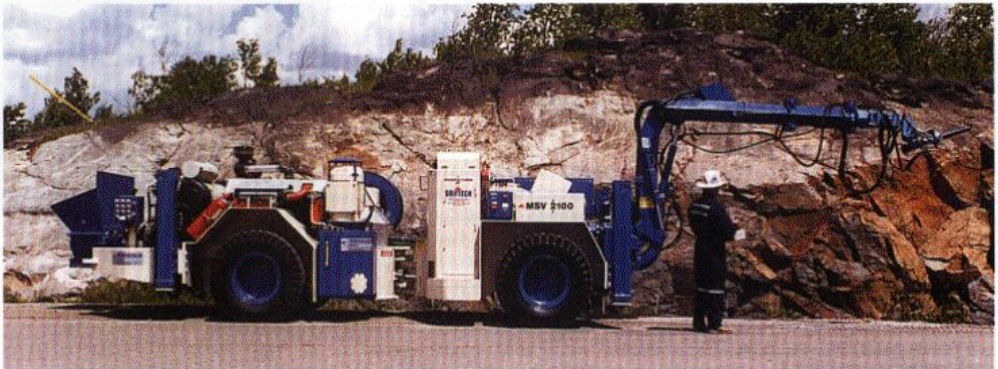
Figure 3. Underground mining shotcrete sprayer.
