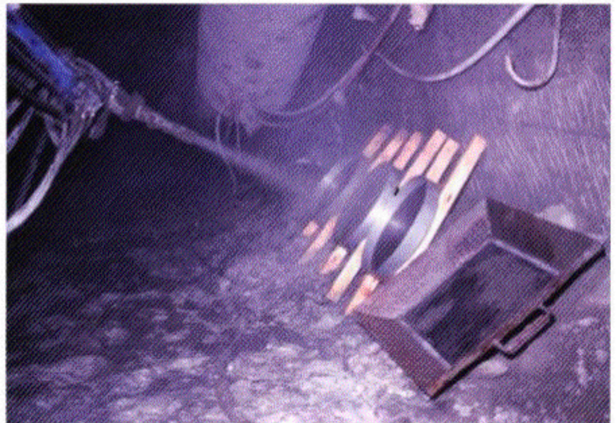
Figure 3. Specimen production in an underground environment.
