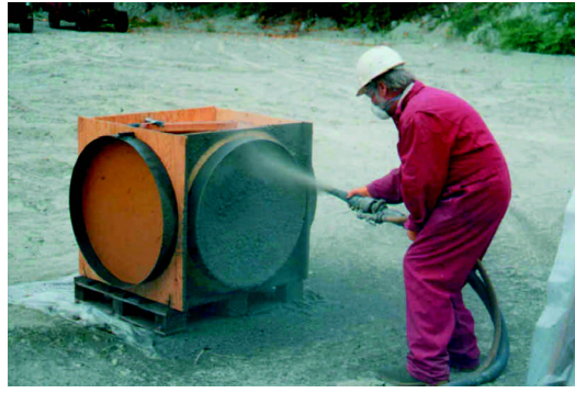
Figure 5. Shooting of a round panel with fiber-reinforced shotcrete for testing using the proposed new ASTM centrally loaded round determinate panel test.
