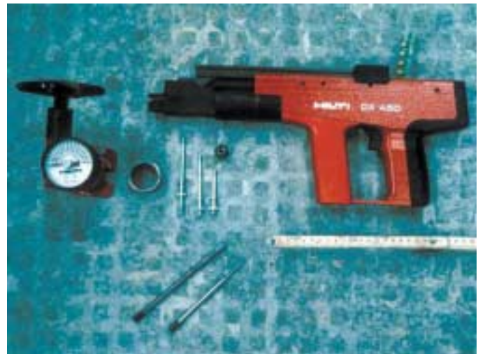
Figure 6: Testing equipment for stud-driving method.
