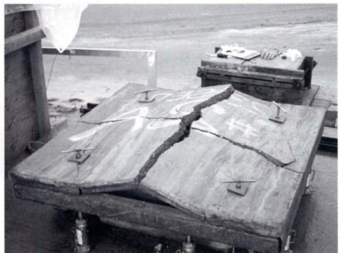
Figure 2. Steel fiber reinforced shotcrete panel at 150 mm (5.6 in.) deflection.
