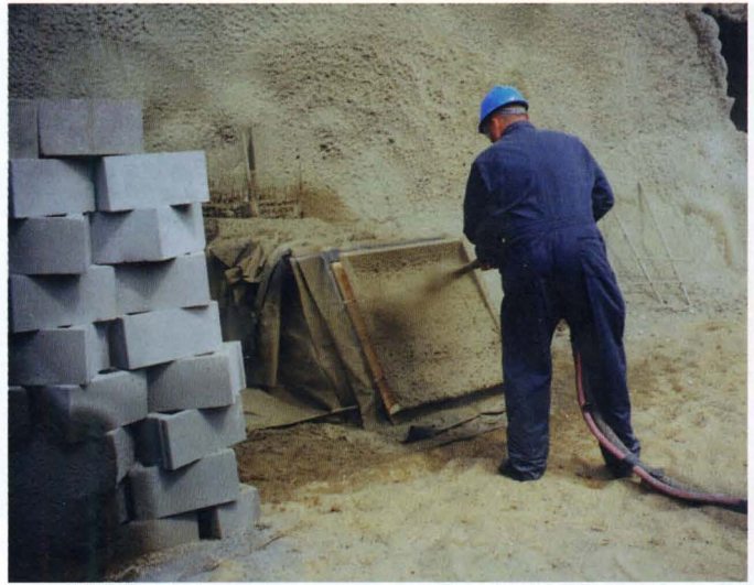
Nozzleman candidate completes wet-mix vertical test panel
