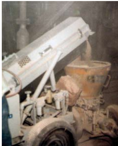
Predampener feeding material to a rotary gun
